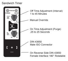
Sandwich CRT - Adjust the timer by turning the dimple in the adjustment wheel to correspond to the numerical number value on the timer bezel.
