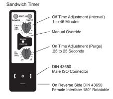
Sandwich CRT - Adjust the timer by turning the dimple in the adjustment wheel to correspond to the numerical number value on the timer bezel.
