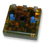
Canfield Connector also has the capability to offer Low Pressure Injection Molding (LPIM) with contract overmolding of circuit boards and other more fragile parts. This process is newer in the market place and allows us to fill a specific product need to many customers.
