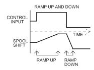
7. Dither - The B5950 uses sine wave dithering with control of frequency (30-150 Hz.) and amplitude (0-.5 A. P-P). Sine wave dithering is sophisticated and allows for smooth control. The **Dither Freq** and **Dither Amp** adjustments on the B5950 are left at some intermediate setting for frequency and at maximum amplitude when the units are shipped. Typically a Dither Frequency of approximately 50 Hz. gives satisfactory operation.
